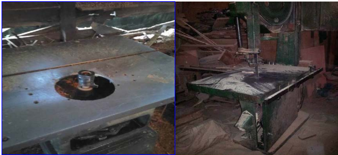
Figure 5.15 A photograph showing a spindle moulder and wood cutter machine regularly used without properly fixed guards exposing site workers to the blade
