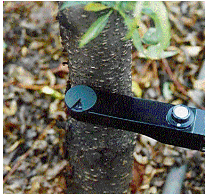
Figure 2.19. View of LAI-2000 Plant Canopy Analyser (PCA) optical sensor with 45° view cap to blank out 315° field-of-view.
