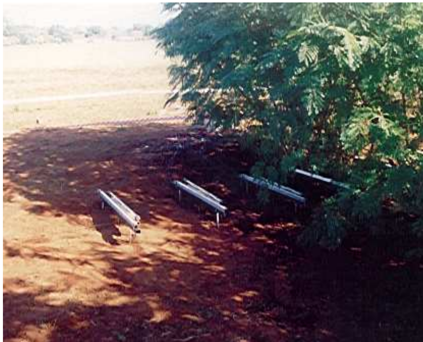
Figure 2.15. View of Leucaena N-S axis hedgerow and tube solarimeters. This is with full canopy ( LAD = 1.55 \text{ m}^2 \text{ m}^{-3} ) with afternoon sunshine.
