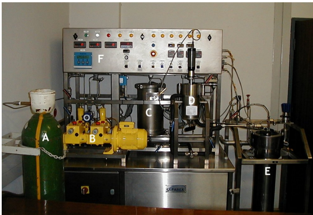
Figure 3.1: A 1l PGSS reactor (Separex Equipments, France) used for encapsulation of bacteria, situated at the Polymers and Ceramics centre, CSIR, Brummeria, PTA. A= CO 2 supply, B= Pump, C= CO 2 preheater, D= Mixing chamber, E= Product chamber, F= Control panel
