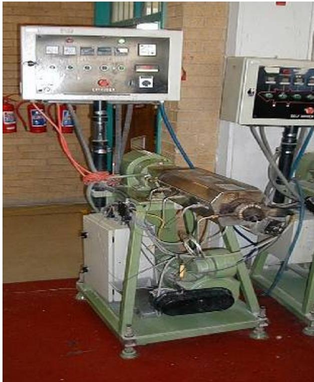
**Figure 11: Rapra single-screw extruder**
