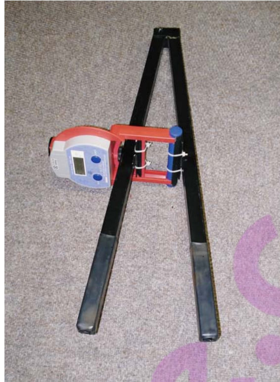
Photo 3.11: Adduction bars with grip dynamometer in place (ready for use)
