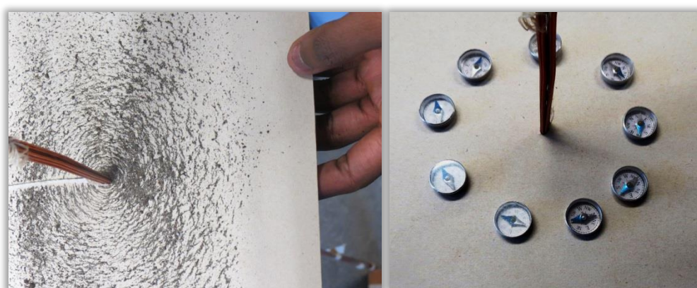
Figure 4-8: Magnetic field around a straight current-carrying conductor
