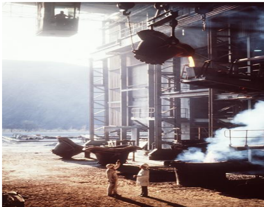
Figure 4.17 An example of particulate emissions inside a Smelter (furnace and converter building) (Impala Platinum, 2001c)
