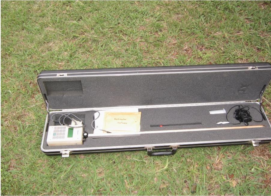
**Figure A3 The sunfleck ceptometer, model AccuPAR, used to measure PAR.**
