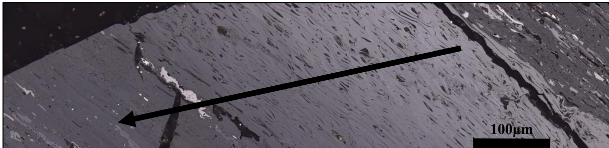
Figure 2.7: Mosaic photomicrograph showing fusinite (right; well-preserved structure, high reflectance) grading into semifusinite (structured still, lower reflectance), and finally into vitrinite (bottom left; unstructured, lowest reflectance) observed in the inertinite-rich sample. 500x magnification, reflected light under oil immersion. Scale is indicated.
