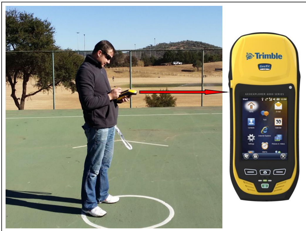
Figure 3.4: Trimble's GeoExplorer 6000 series handheld (model: GeoXH 3.5G) GPS device (Copyright © Trimble Navigation 2014)
