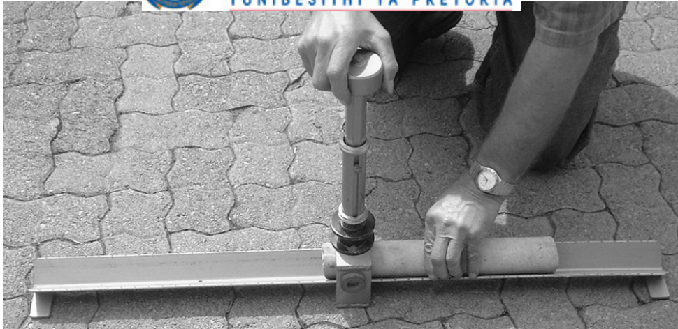
Figure 5-3 The Impact splitting equipment
