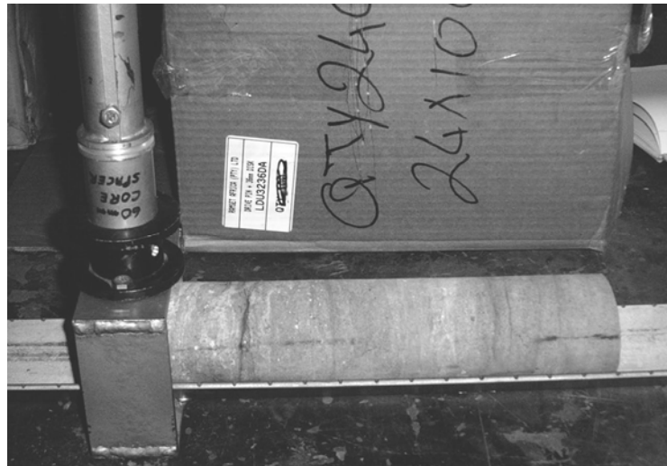
Figure 5-5 A fine to medium grained sandstone or “grit” unit before impact splitting, taken from borehole ARN 4968
