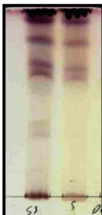
Figure 2.5. Hexane fraction of G. biloba from the solvent-solvent extraction procedure (left) and from the direct extraction procedure (right) sprayed with vanillin with mobile phase DCM: methanol (9:1)
