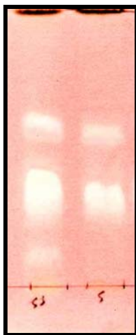
Figure 2.6. Hexane extract and fraction of G. biloba from the solvent-solvent extraction procedure (left) and from direct extraction procedure (right) sprayed with S. aureus and mobile phase DCM: methanol (19:1)
