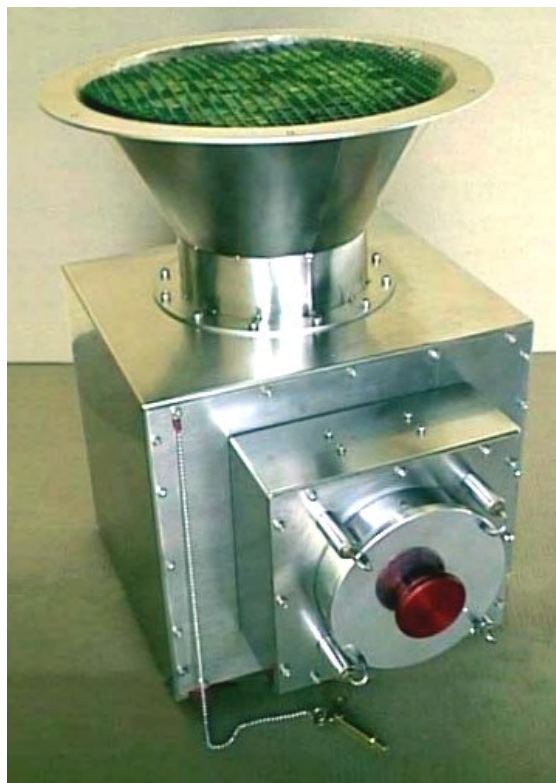
Figure 5.1. The Kotzé Inoculum Monitor illustrating the position of the prepared leaf grid in the hopper (Courtesy of T.N. Janse van Rensburg).
