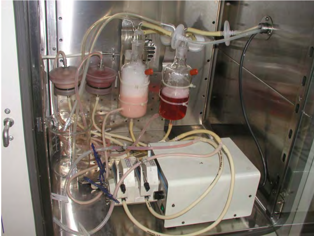
Figure 4.3.1 The dual bioreactor in vitro model/s of the BALSS. The PFC reservoir and bioreactor are on the left (pink). The PFC(-) medium reservoir and bioreactor are on the right (red). Compare this configuration with the earlier single version (figure 4.2.1 above).
