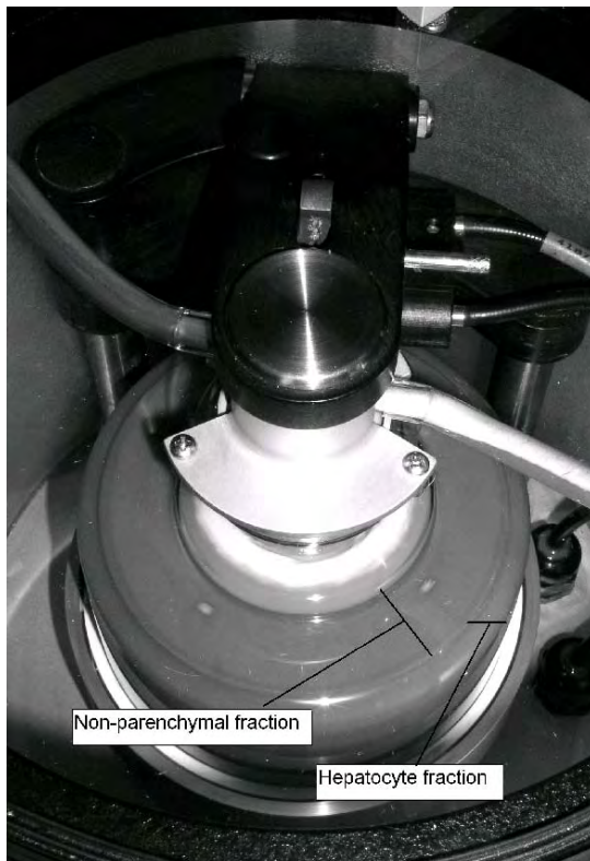
Figure 4.1.6b BRAT Bowl after addition of Percoll. Separation has occurred.
