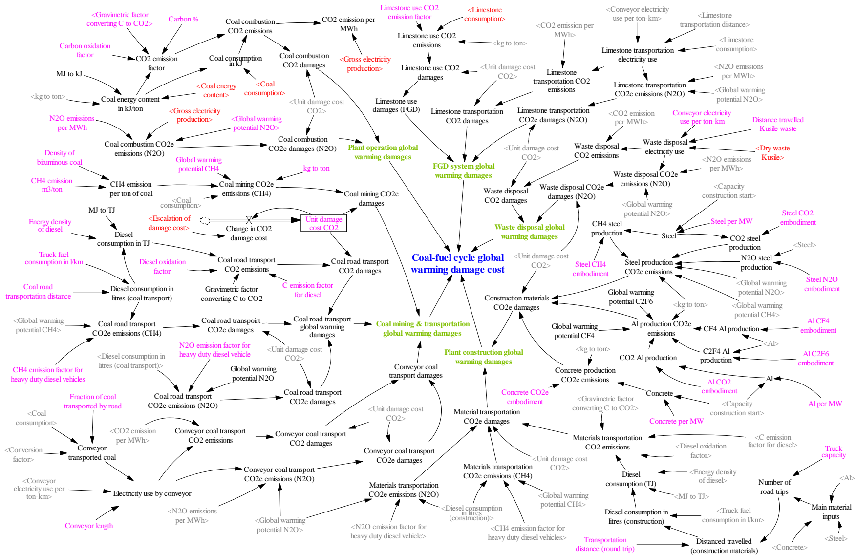
Figure 6.10: Global pollutants sub-model stock and flow diagram
