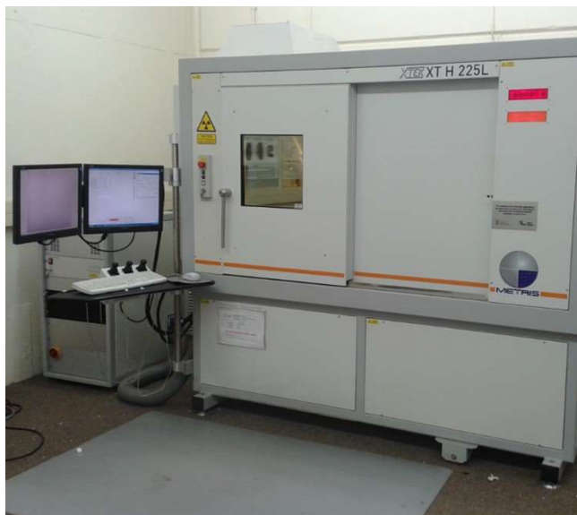
Figure 4.6. Nikon XTH/225-ST Microfocus X-ray microtomography system
