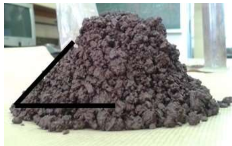
Figure 3.5. Angle of repose for granulated mixtures where granules are sticky
