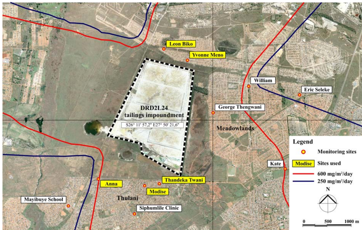
Figure 122: Dust fallout monitoring sites in the vicinity of the DRD tailings impoundment. Predicted total daily average dust fallout ( \text{mg}/\text{m}^2/\text{day} ) from the DRD tailings impoundment.
