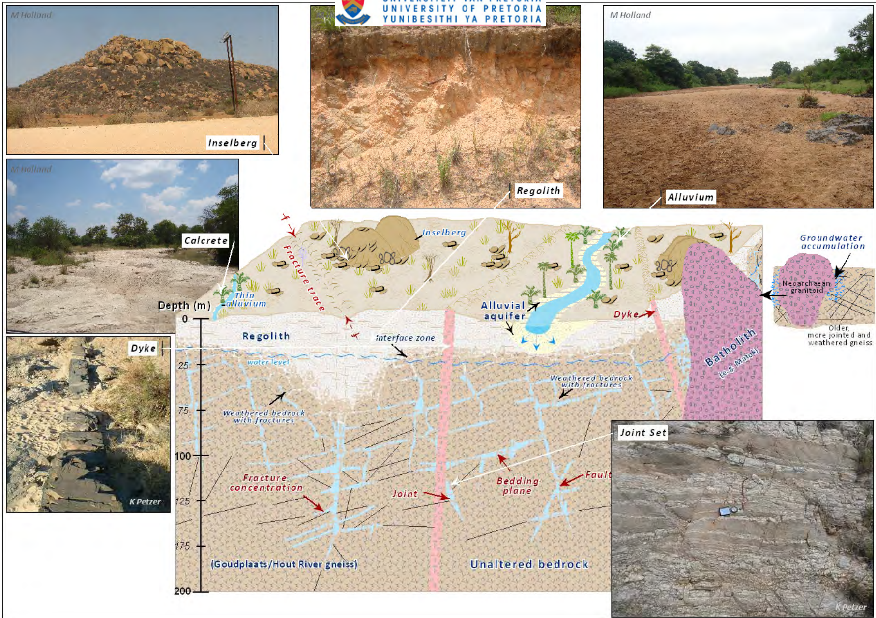
Figure 4.12. Generalised section of the aquifer systems found in the area of investigation, including photo's of observed geological features.
