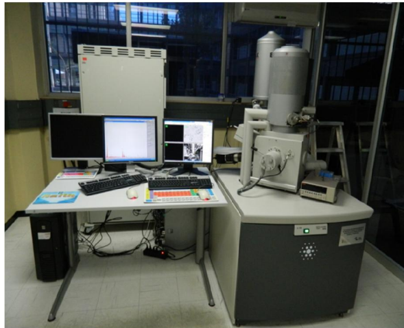
Figure 4.9: The Mintek's FEI NOVA NanoSEM 230 FEG used for EBSD
