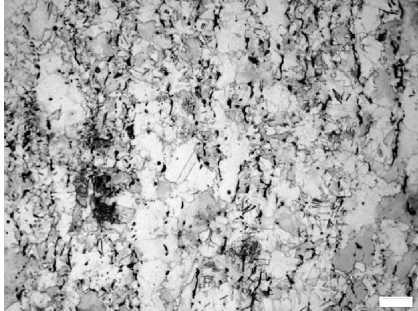
Figure 5.18: Optical micrograph steel 321 after 9 passes at a strain rate of 0.01 \text{ s}^{-1} . The final deformation temperature after the 9 passes was 800^\circ\text{C} . Note the unrecrystallised microstructures. (the scale bar indicated on the figure is 100 \mu\text{m} ).
