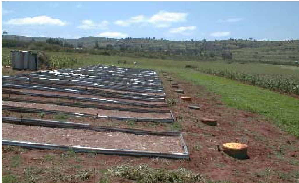
A. Experimental setup of the runoff plots
