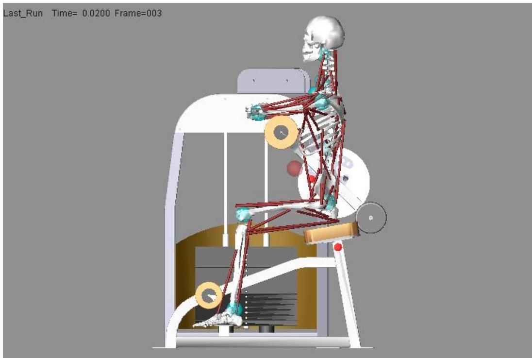
**Figure 1: 3D musculoskeletal modelling of the abdominal crunch resistance training machine and 95<sup>th</sup> percentile male musculoskeletal model using LifeModeler™ and MSC ADAMS software.**
