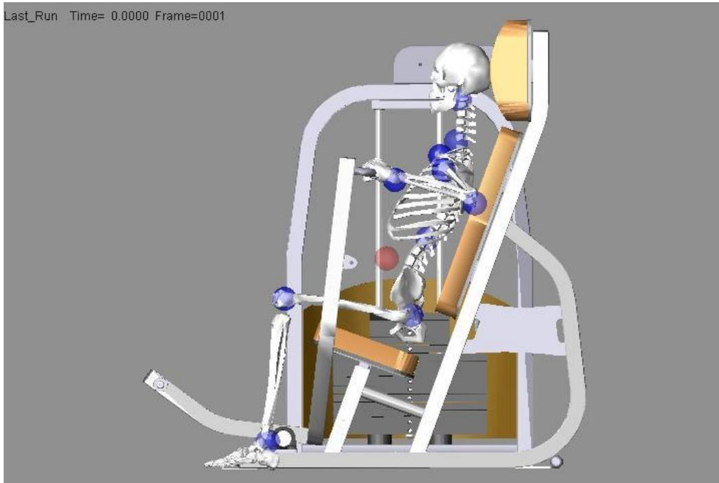
**Figure 1. 3D musculoskeletal modelling of the chest press resistance training machine and 95<sup>th</sup> percentile male musculoskeletal model using LifeModeler™ and MSC ADAMS software.**
