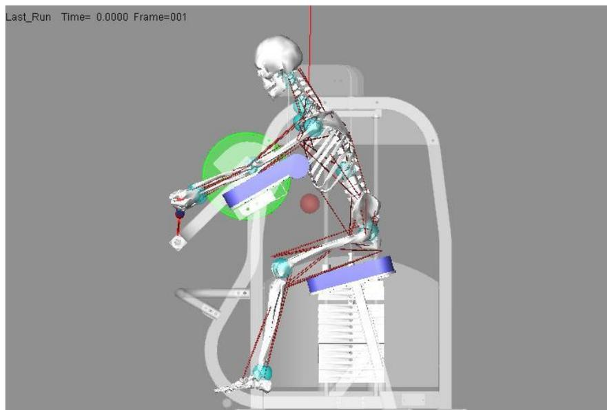
**Figure 1. 3D musculoskeletal modelling of the biceps curl resistance training machine and 50<sup>th</sup> percentile male musculoskeletal model using LifeModeler™ and MSC ADAMS software.**
