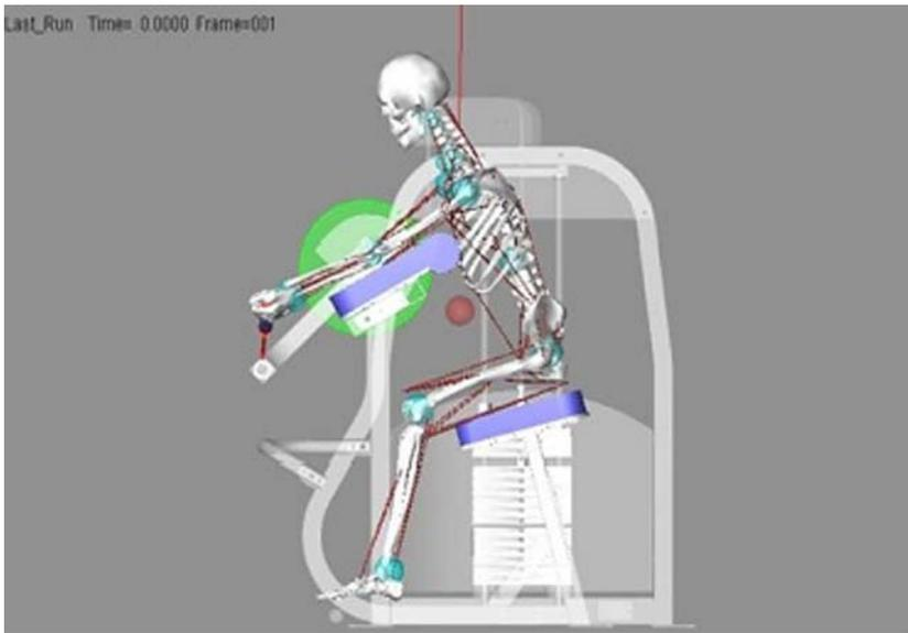
Figure 1. 3D musculoskeletal modelling of the biceps curl resistance training machine and 50<sup>th</sup> percentile male musculoskeletal model using LifeModeler™ and MSC ADMAS software.
