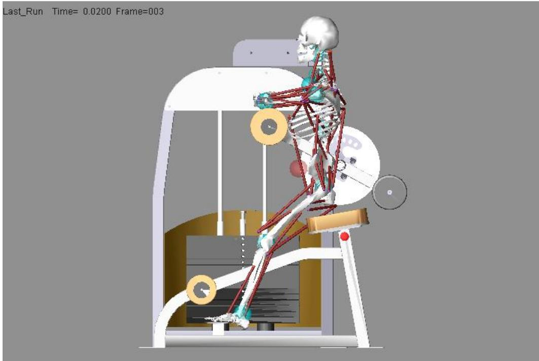
**Figure 8. 5<sup>th</sup> percentile female's positioning on the abdominal crunch resistance training machine**
