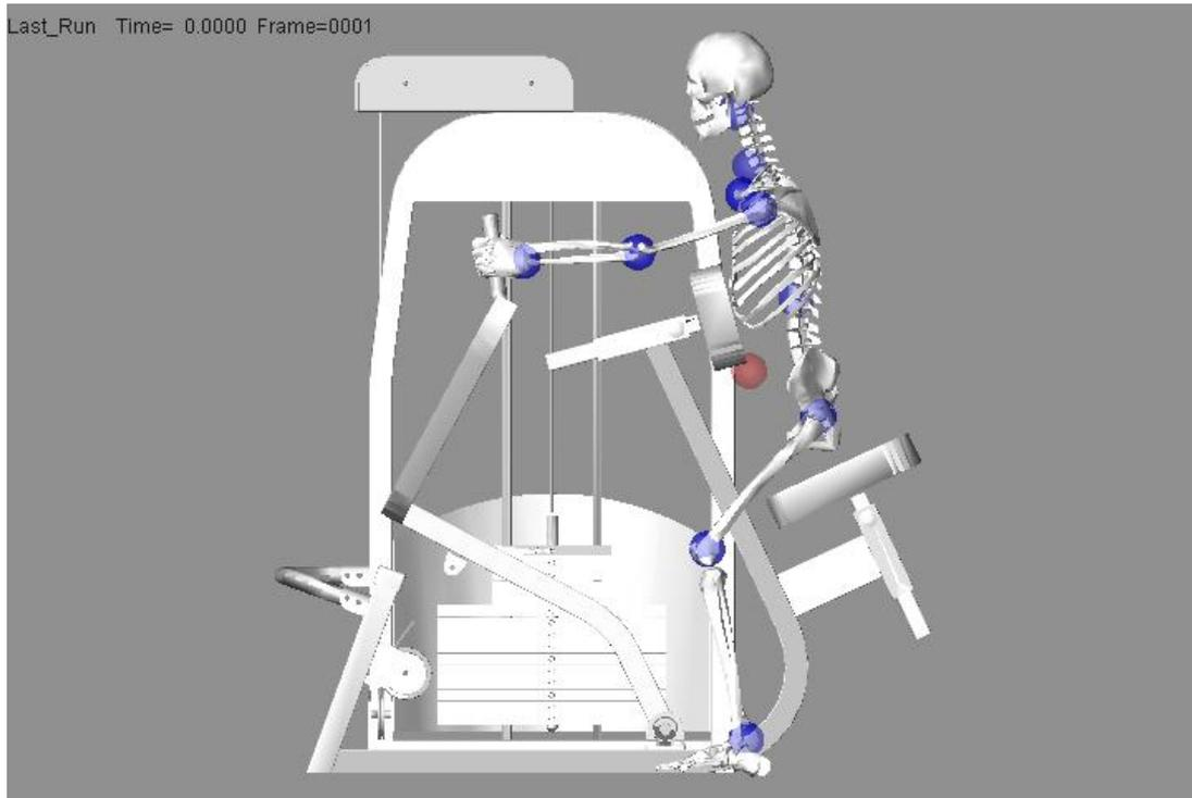
**Figure 1. 3D musculoskeletal modelling of the seated row resistance training machine and 50<sup>th</sup> percentile male musculoskeletal model using LifeModeler™ and MSC ADAMS software.**
