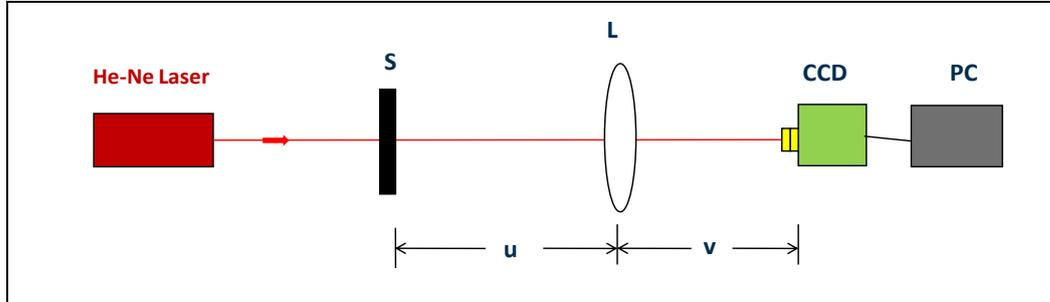
Figure 3.10: Experimental setup: S (Sample), L (Lens  $f=150\text{mm}$ ,  $D=50.8\text{mm}$ ), CCD (Camera), PC (Computer),  $u$  (Object distance = 450 mm),  $v$  (Image distance = 225 mm),  $F$ = filters,  $M$  ( $v/u$ )= 0.5, HeNe Laser power = 9 mW.
