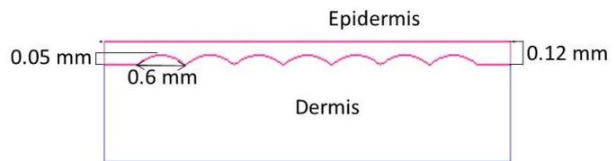
Figure 3.4: Wavy epidermis/dermis interface 0.12 mm into the skin with a wave amplitude of 0.05 mm and length of 0.6 mm.
