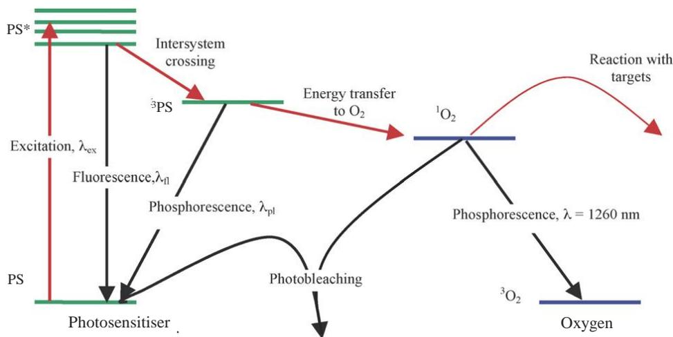
Figure 2.16: Energy level diagram for a Type 2 photosensitiser.
