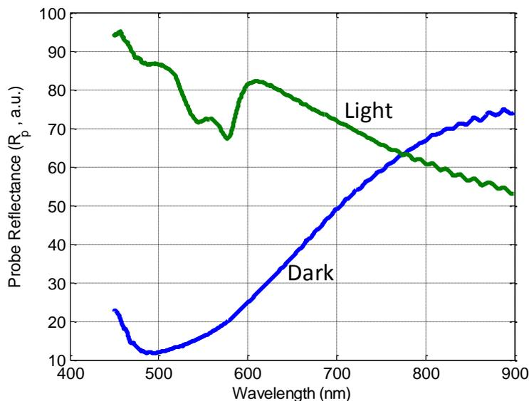
Figure 4.12: Reflectance measurements for two different skin phototypes.
