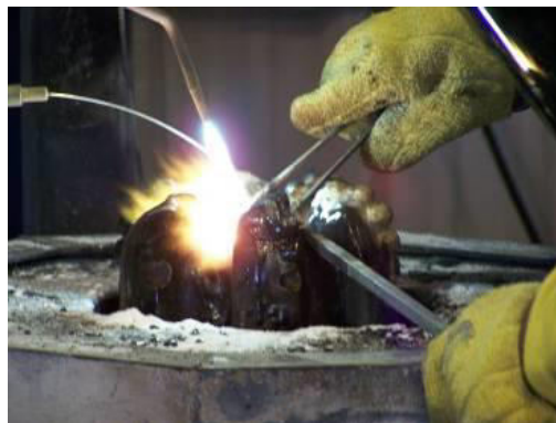
Figure 1.9: Brazing of PCD inserts into a bit [16]
