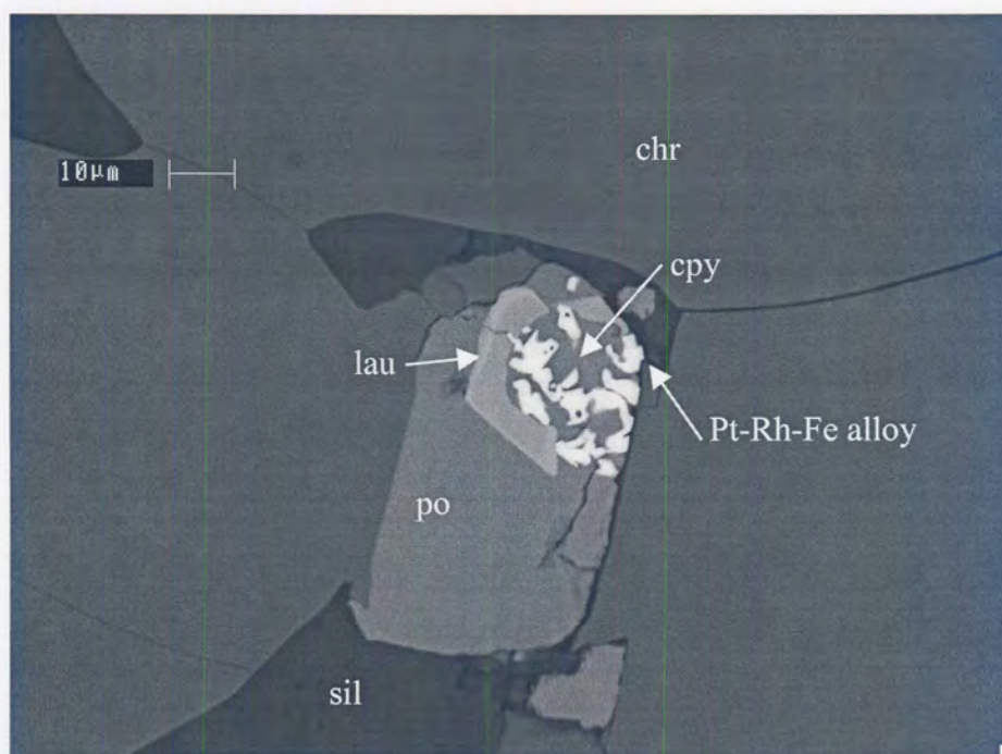
Figure 51 Pt-Rh-Fe alloy (brightest grains) associated with zoned laurite (lau) (the higher backscattered-electron intensity is the result of a higher Os concentration in the rim) included in a composite chalcopyrite (cpy) and pyrrhotite (po) grain at the grain-boundary of silicate (sil) and chromite (chr). Backscattered-electron image.
