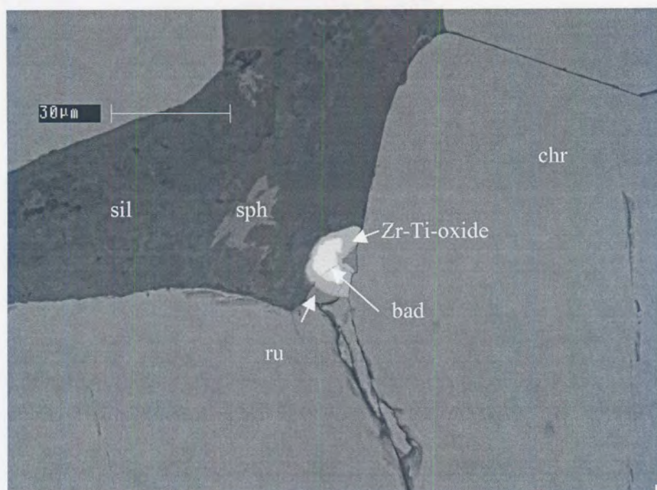
Figure 31 Complex oxide assemblage consisting of baddeleyite ( bad ) (brightest grain) in the centre, rimmed by Zr-Ti-oxide (slightly darker), and rutile ( ru ) at the grain boundary of chromite ( chr ) and a fine-grained intergrowth of secondary hydrous silicates ( sil ) and sphene ( sph ). Backscattered-electron image.
