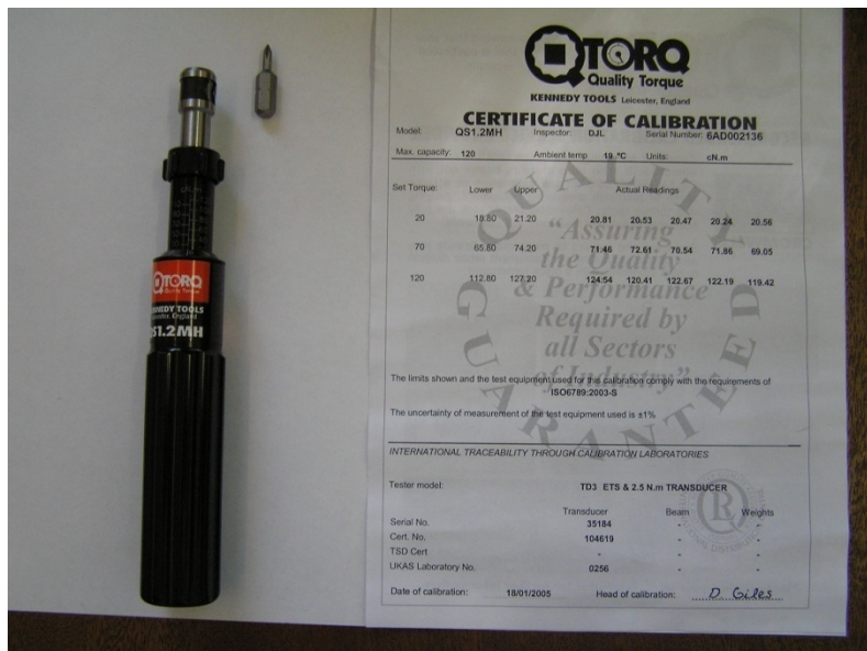
Figure 30: Calibrated torque screwdriver, pre-set at 40 N/cm together with a certificate of calibration
