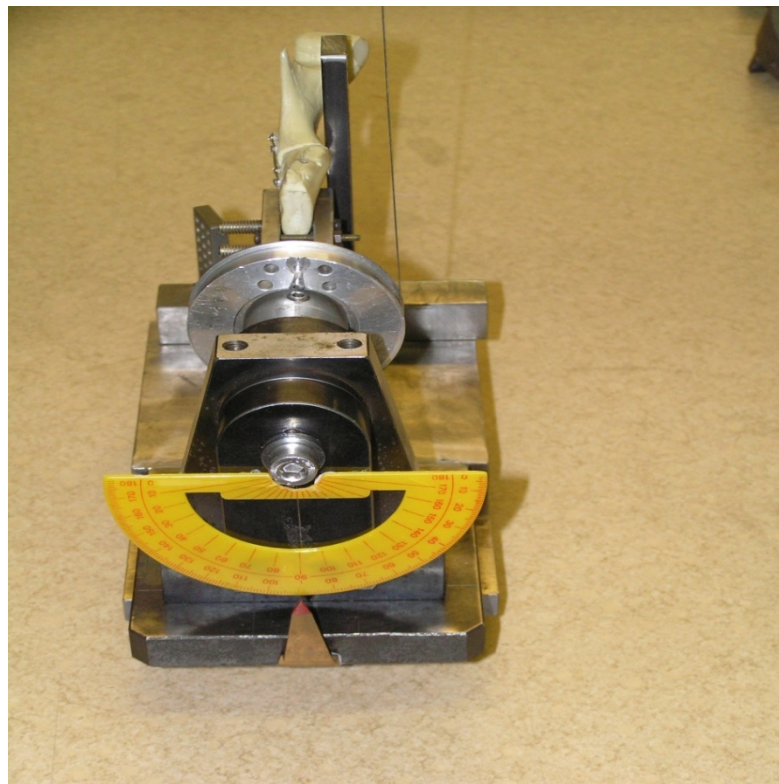
Figure 22: Device used for measuring the degrees of rotation at specific torque applications
