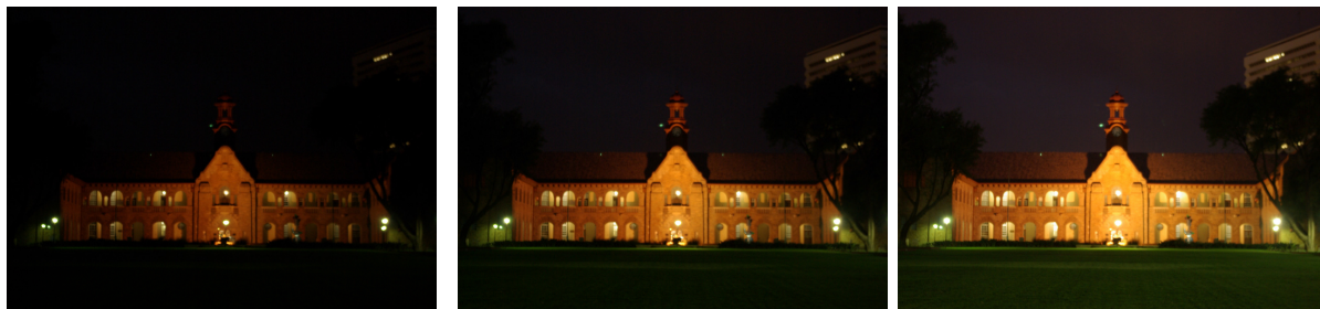
(a) ISO=400, f_{number}=f/5.6 , t_{exposure}=0.5s , f=50mm (b) ISO=400, f_{number}=f/5.6 , t_{exposure}=1.5s , f=50mm (c) ISO=400, f_{number}=f/5.6 , t_{exposure}=3s , f=50mm
