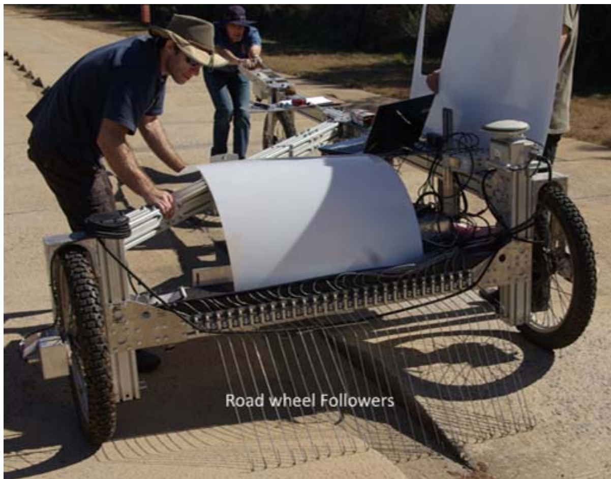
Figure 7.5: CanCan machine using road wheel followers and INS system
