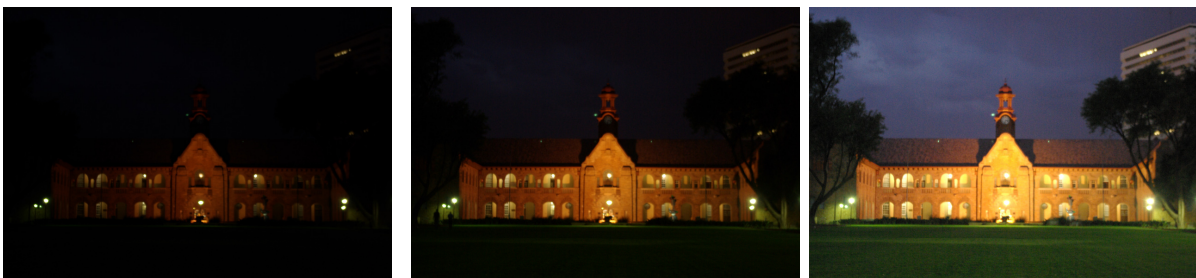
(a) ISO=100 , f_{number}=5.6 , t_{exposure}=1s , f=50mm (b) ISO=400 , f_{number}=5.6 , t_{exposure}=1s , f=50mm (c) ISO=1600 , f_{number}=5.6 , t_{exposure}=1s , f=50mm
