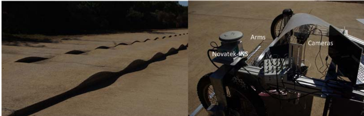
Figure 7.6: Sinusoidal profile. Experimental setup
