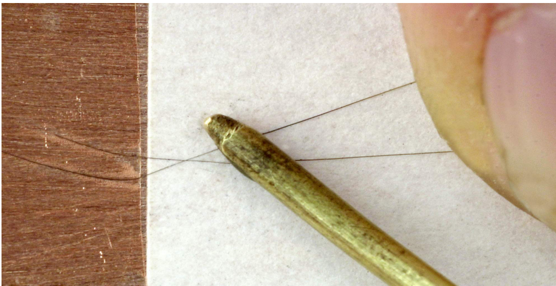
Figure 4-5: Photograph showing how thermocouple wires are positioned for making a thermocouple by spot welding.
