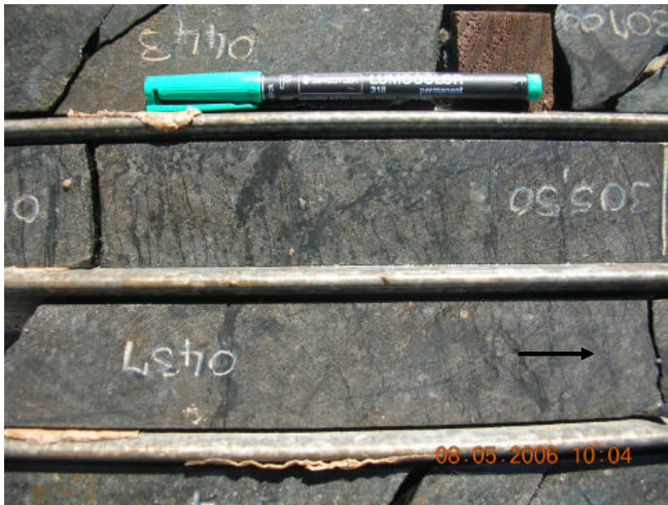
Fig. 3.7: Medium-grained peridotite with serpentine veins at 305.50m depth, borehole 2121. Arrow indicates stratigraphic up. Pen is shown for scale.
