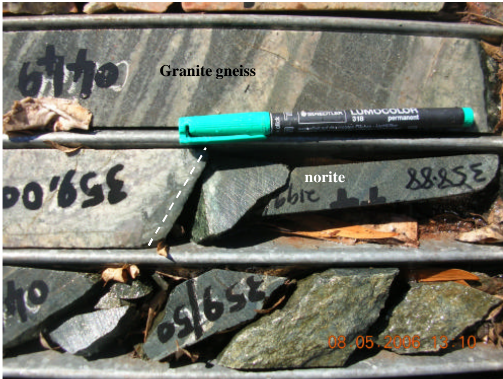
Fig. 3.17: Granite gneiss in sharp contact (at 359.00 m) with fine-grained (chilled) norite. Stippled line represents the contact. Pen included for scale. Borehole 2199.
