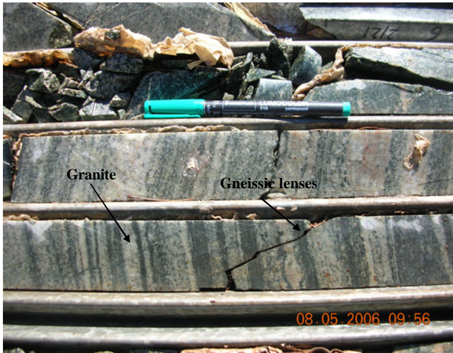
Fig. 3.3: Medium-grained, pinkish-grey granite gneiss containing dark green melanosomes that define rhythmic layering. 330m depth, borehole 2121. Pen is shown for scale.
