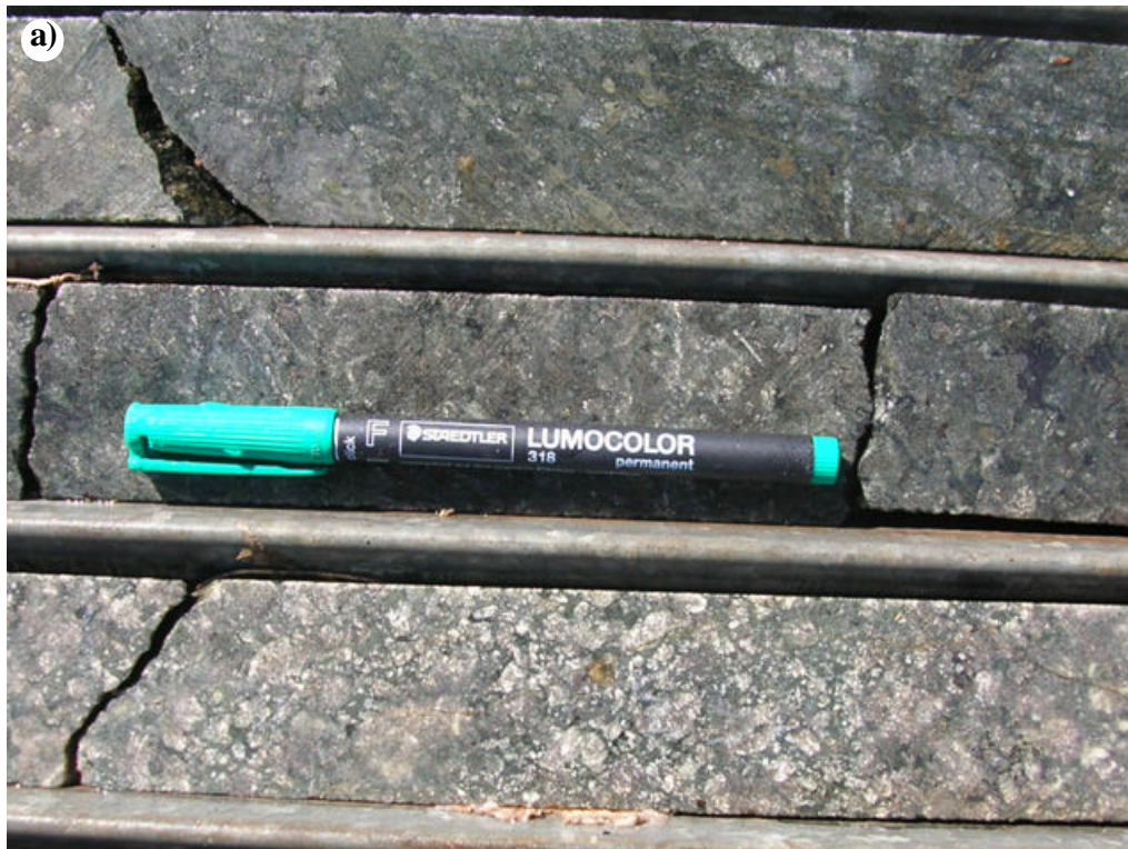
Fig. 3.15a: leucocratic gabbro-norite at the base of the Main Zone at 171.50m depth, borehole 2121. Stratigraphic up direction is towards the top of the page. Pen is shown for scale.
