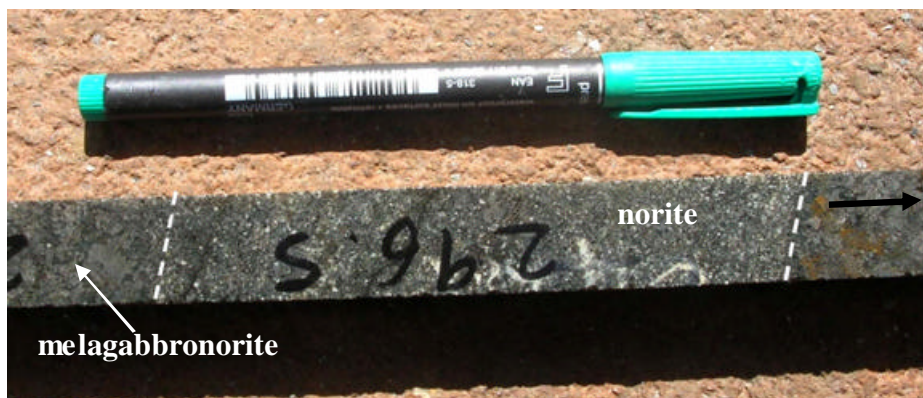
Fig. 3.6: Sharp contact (at 296.62 m and 296.50 m depth) between medium-grained, sulphide-bearing melagabbronorite and fine-grained, poorly mineralized to barren norite. Stippled lines represent the contact. Arrow indicates stratigraphic up. Pen is shown for scale. Borehole 2121.
