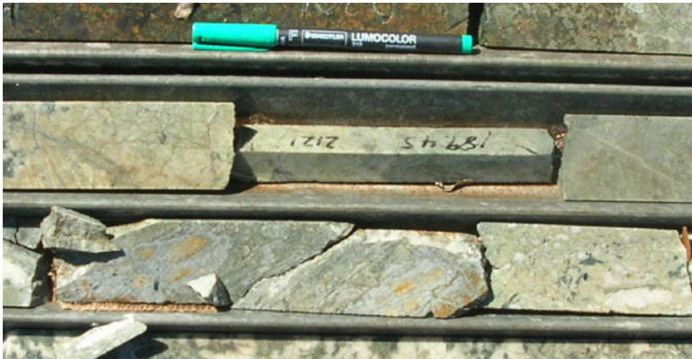
Fig. 3.14: Dolomite xenolith separating Platreef and Main Zone at 197.47m depth, borehole 2121. Pen is shown for scale.
