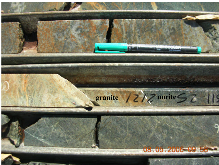
Fig. 3.4: Sharp contact at 311.30m depth (indicated by stippled line) between granite gneiss (above) and fine-grained (chilled) norite (below). Pen is shown for scale. Borehole 2121.
