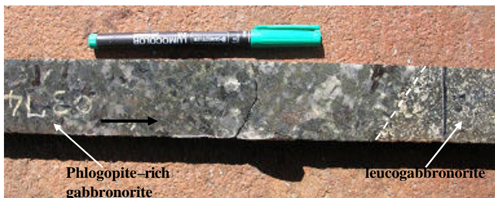
Fig. 3.10: Phlogopite-rich gabbronorite in contact (at 274.15m depth) with leucogabbronorite. Note the sharp contact between the two rock types. Stippled line represents the contact. Arrow indicates stratigraphic up. Pen is shown for scale. Borehole 2121.
