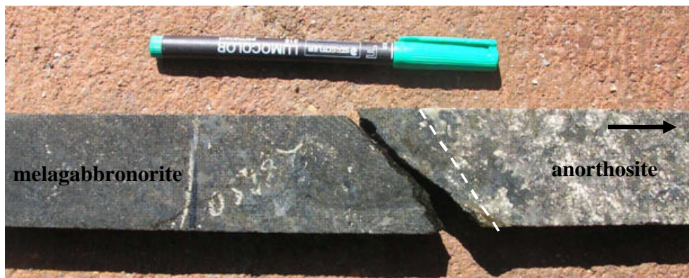
Fig. 3.9: Anorthosite in contact (at 281.42m depth) with fine-grained melagabbronorite. Note the sharp contact between the two rock types. Arrow indicates stratigraphic up. Stippled line represents the contact. Pen is shown for scale. Borehole 2121.
