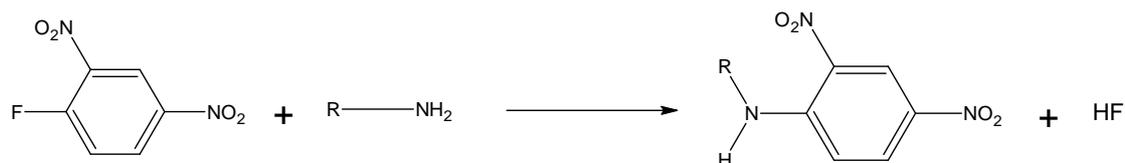
**Figure 3.18** Reaction scheme for the reaction of 2, 4-dinitrofluorobenzene (DNFB) with a primary amine. R = alkyl or aryl substituent [121].
