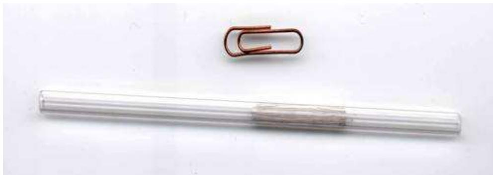
**Figure 2.9** A polydimethylsiloxane multichannel trap (PDMS MCT). This trap has 32 x ~2 cm lengths of PDMS tubes arranged in parallel inside a glass tube. This shorter arrangement is suitable for trapping less volatile analytes which require longer desorption times.
