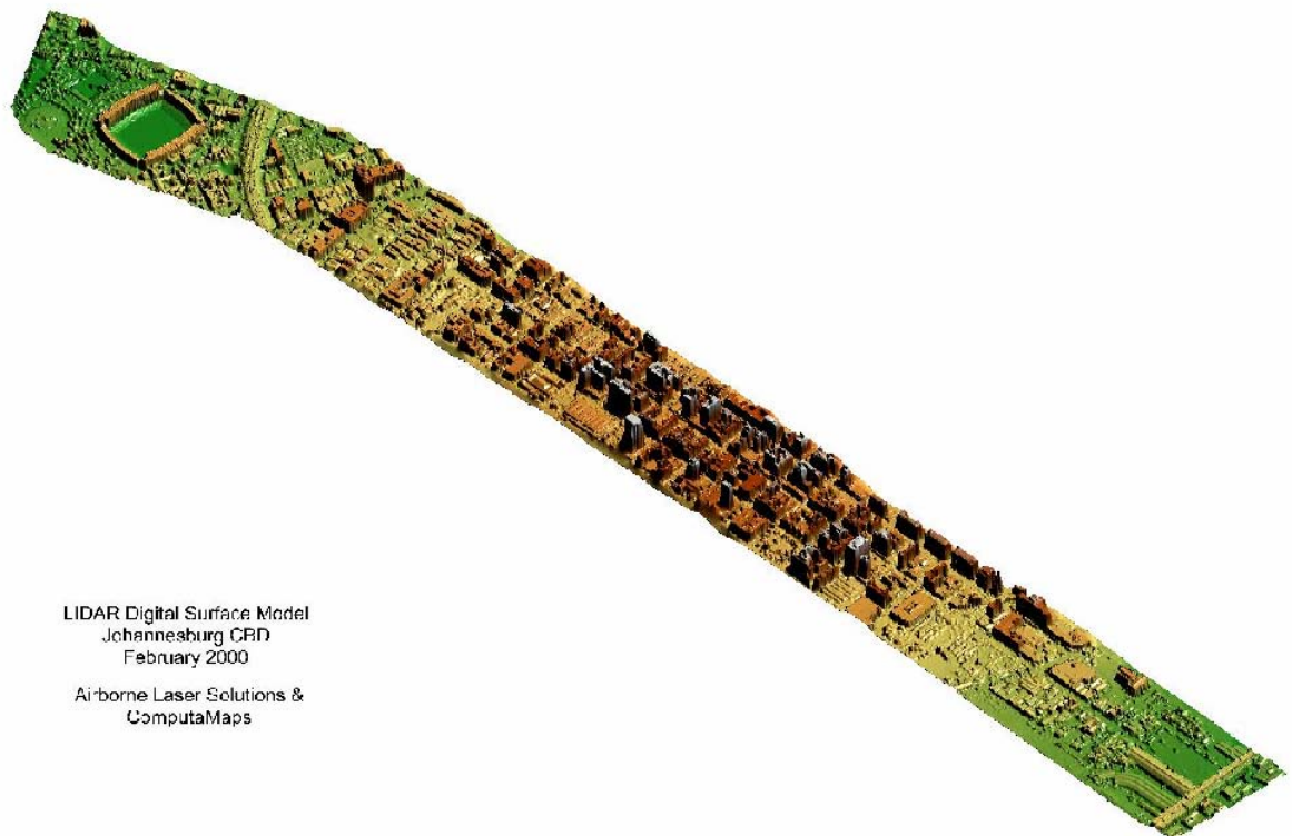
Figure 3.11: LiDAR digital surface model over Johannesburg CBD
