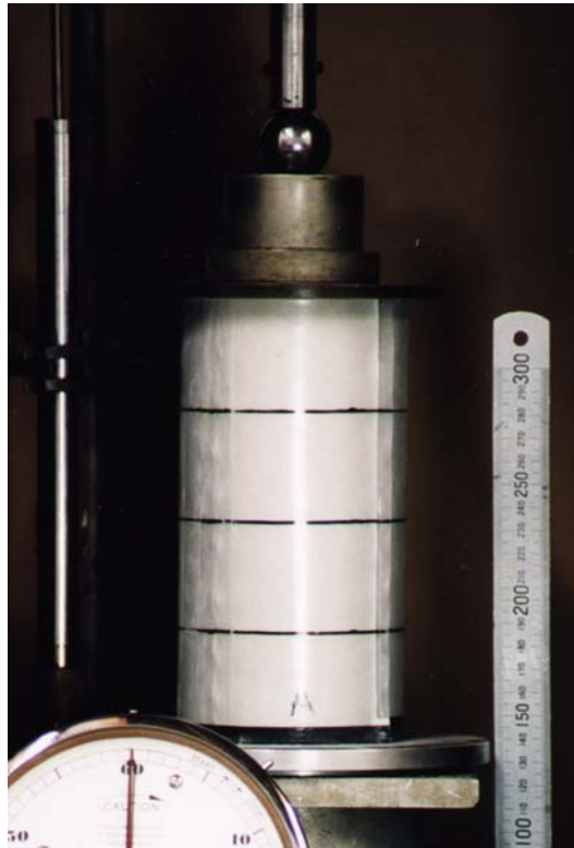
Figure 3.31 Single cell specimen in test machine.
