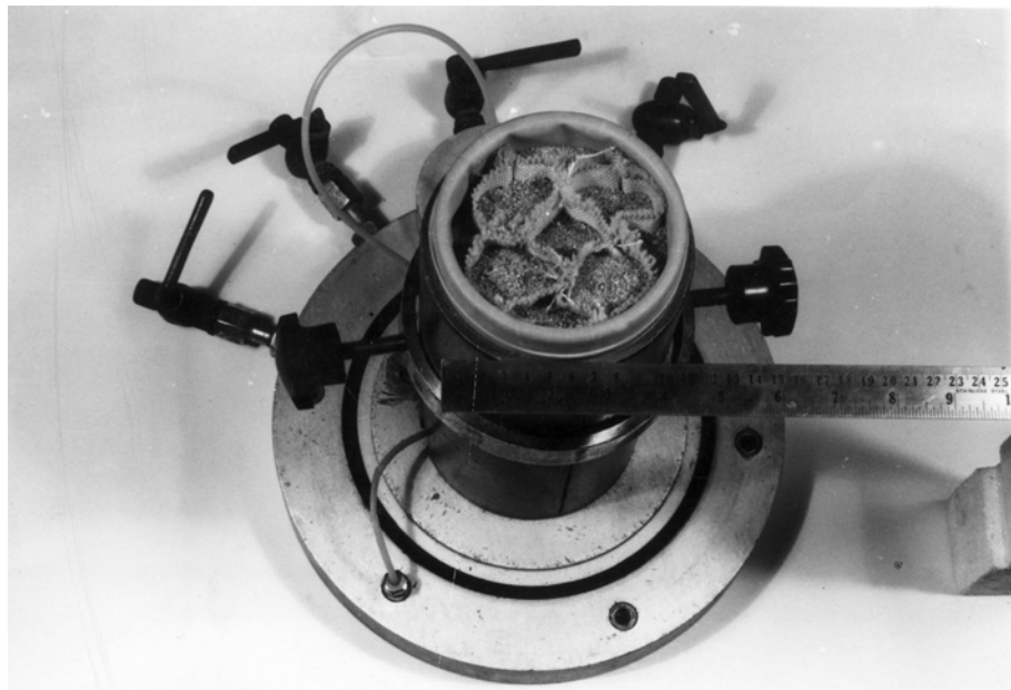
Figure 2.17 Triaxial test sample with four interconnected cells tested by Rajagopal et al. (1999).
