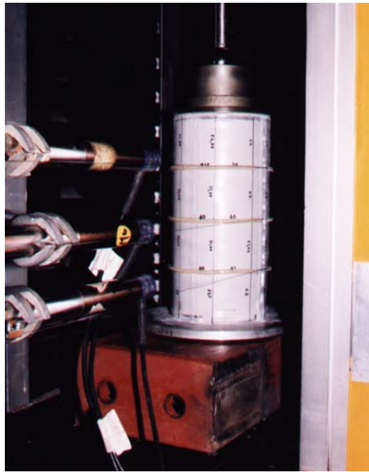
Figure 3.29 Instrumentation for measuring the circumferential strain of the specimens.
