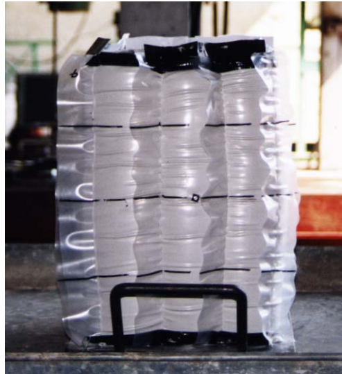
Figure 3.41 The 3x3 cell pack after compression.
