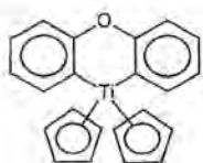
Bis(cyclopentadienyl)(diphen-2,2'-yl ether)titanium(IV) [TiCp 2 (Dpe)] 2-11
