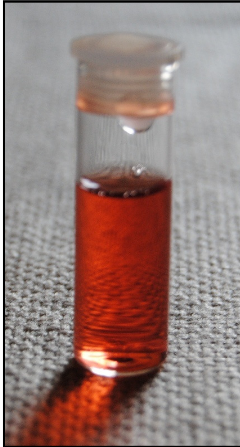
Figure 6.5. Photograph of diluted Riminocelles The distinctive red colour is evidence that (non-water-soluble) B663 has been solubilised in an aqueous dispersant through encapsulation within micelles.
