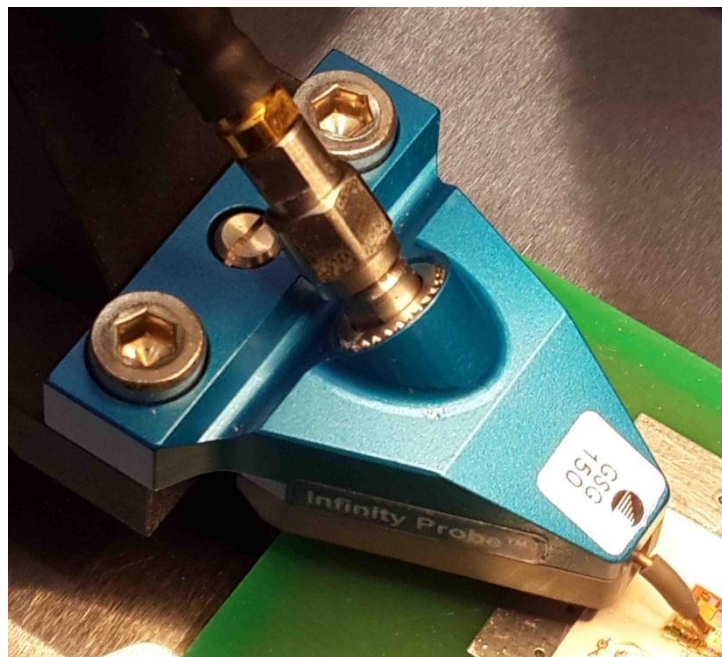
Figure 3.7. The i110 GSG Infinity probe.
