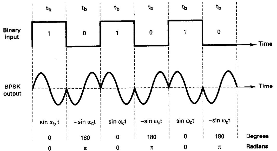
FIGURE 12-17 Output phase-versus-time relationship for a BPSK modulator
