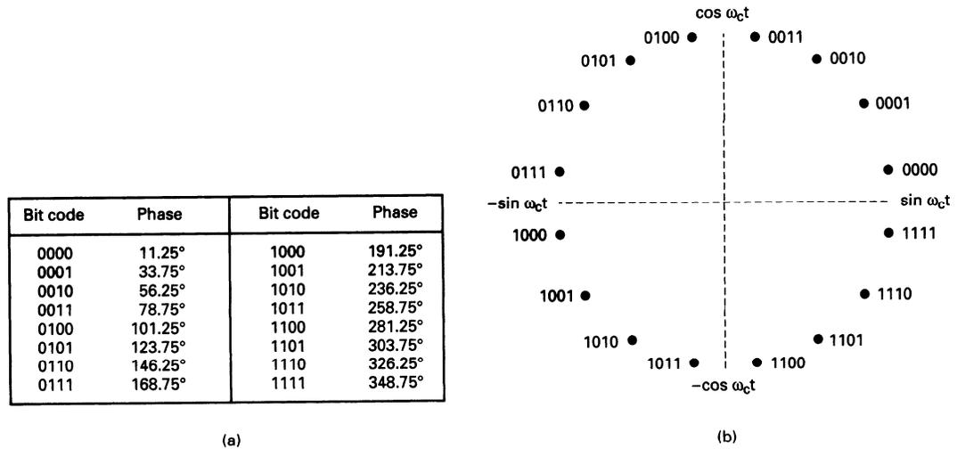
FIGURE 12-31 16-PSK: (a) truth table; (b) constellation diagram
