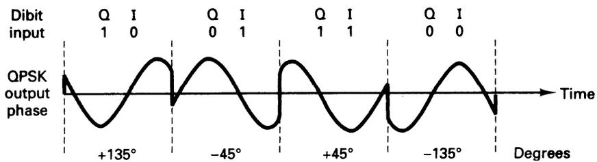
FIGURE 12-21 Output phase-versus-time relationship for a QPSK modulator
