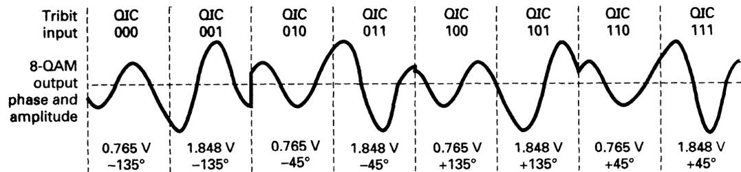
FIGURE 12-34 Output phase and amplitude-versus-time relationship for 8-QAM
