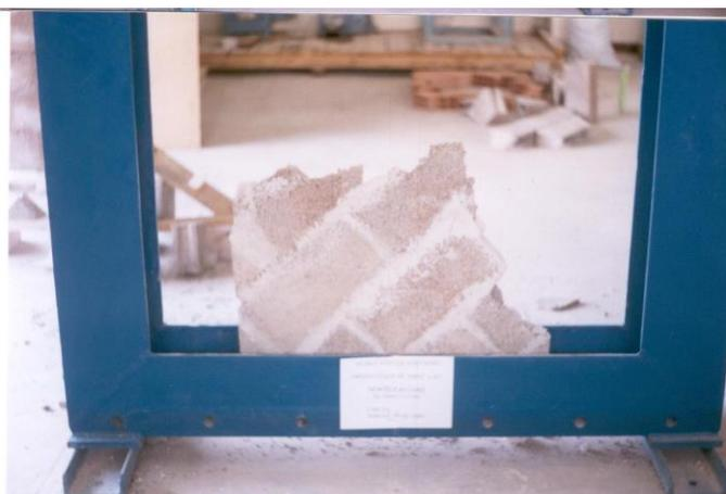
Photo 5.5 Mode de rupture du parpaing ( $\theta = 45^\circ$ )
