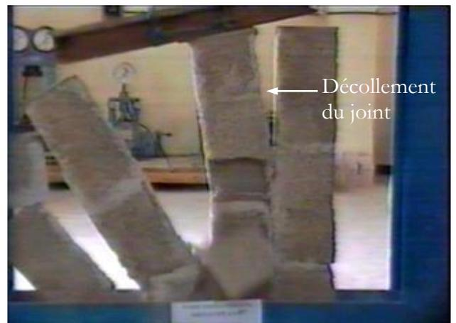
Photo 5.6 Mode de rupture du parpaing ( $\theta = 0^\circ$ )
