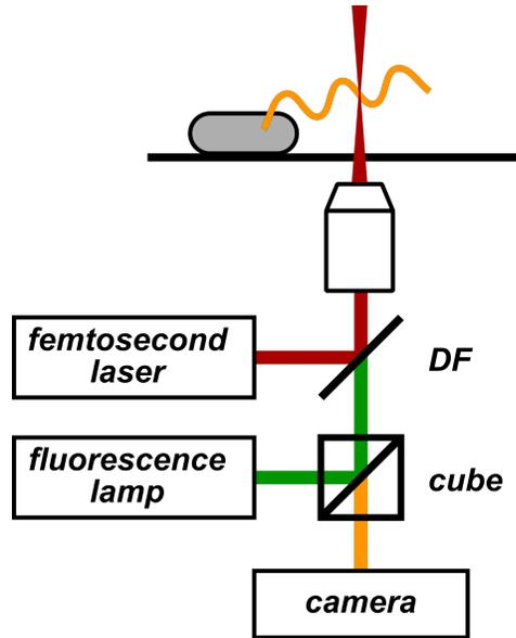
FIGURE 2.1 – Schematic of the experimental setup. The femtosecond laser is added to the optical axis through a dichroic filter (DF) and focused on the sample with a 100X 1.3 NA objective. The same objective is used for fluorescence imaging. The sample is illuminated with a broadband light source and a fluorescence cube selects the excitation and emission wavelengths. The bacterial filaments are then visualized on an EMCCD camera. Every figure in this chapter is taken from [41]
