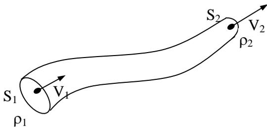
$$Q_m = Q_{m1} = Q_{m2} = \rho_1 V_1 S_1 = \rho_2 V_2 S_2$$
