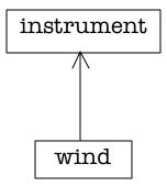
Casting from derived to base moves *up* on the inheritance diagram, so it's commonly referred to as upcasting. Upcasting is always safe because you're going from a more specific type to a more general type — the only thing that can occur to the class interface is that it lose methods, not gain them. This is why the compiler allows upcasting without any explicit casts or other special notation.
