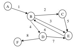
Each state is shown as a circle containing the name of the state, and the input that causes the state to change from one circle to another is indicated next to the arrow showing the direction of change. Thus, if you're in state B and the input is 3, the machine changes to state E.
