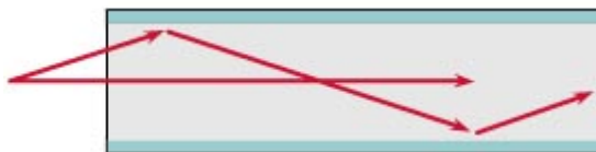
Figure 4.8 : la fibre multimode
