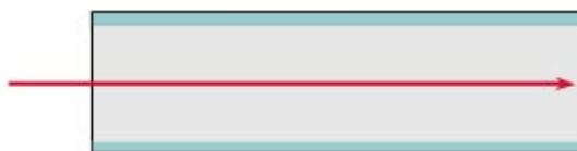
Figure 4.7 : la fibre monomode
