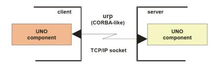
Figure 4: Communication between two UNO components [Flat02]
