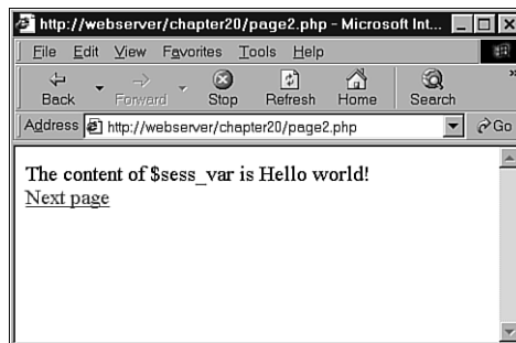
Figure 20.2 The value of the session variable has been passed along via the session ID to page2.php.
