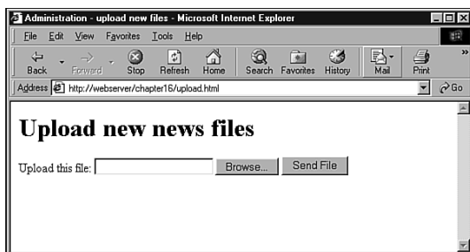
Figure 16.1 The HTML form we use for file upload has different fields and field types from those of a normal HTML form.
