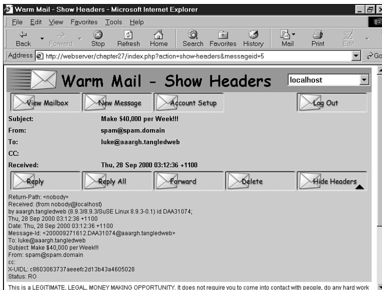
Figure 27.7 Using show-headers to see the full headers for this message will help a user track down the source of the spam.
