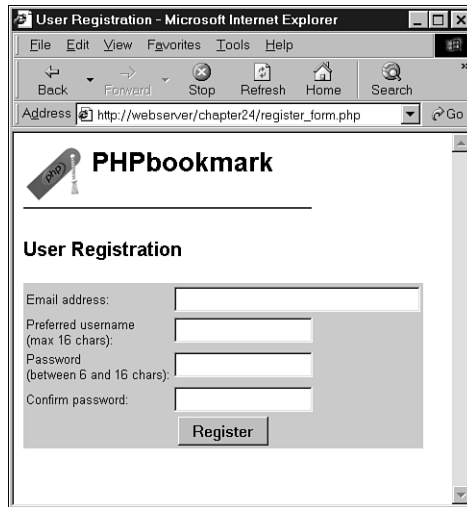
Figure 24.4 The registration form retrieves the details we need for the database. We get users to type their passwords twice, in case they make a mistake.
