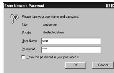
Figure 13.2 Web browsers prompt users for authentication when they attempt to visit a restricted directory on a Web server.
