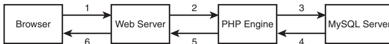
Figure 7.9 The basic Web database architecture consists of the Web browser, Web server, scripting engine, and database server.
