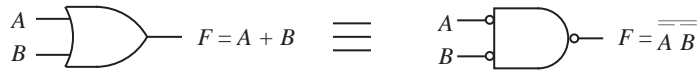
Figure A-13 DeMorgan's theorem is used in mapping an OR gate onto a NAND gate.
