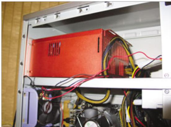
Just about every tower-style PC has its power supply located in the upper-rear corner of the system's case.
