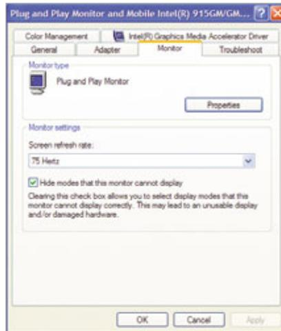
**Upping the refresh rate on your CRT (cathode-ray tube) monitor can eliminate flickering.**
