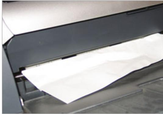
A common cause of printer errors is a simple paper jam.
