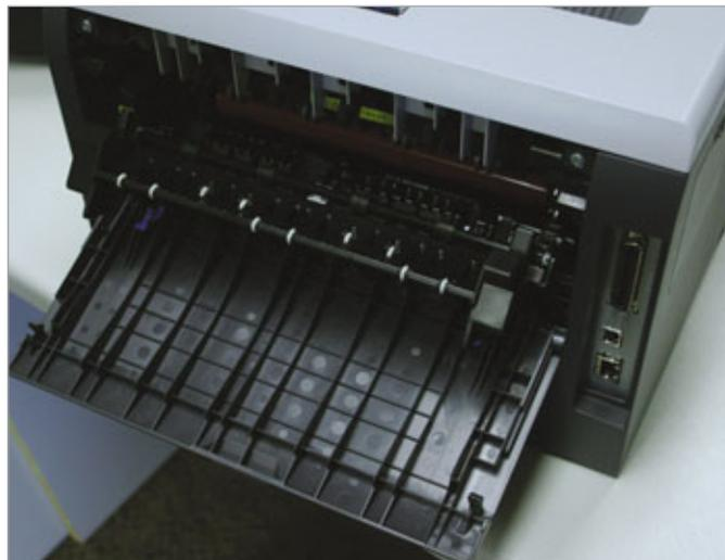
Laser printers often feature a removable rear panel to reach paper jams in the fuser mechanism at the back the printer.
