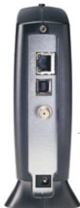
Without a reset button, you can simply unplug the power cable and the PC connection cable from your modem to reset it.
