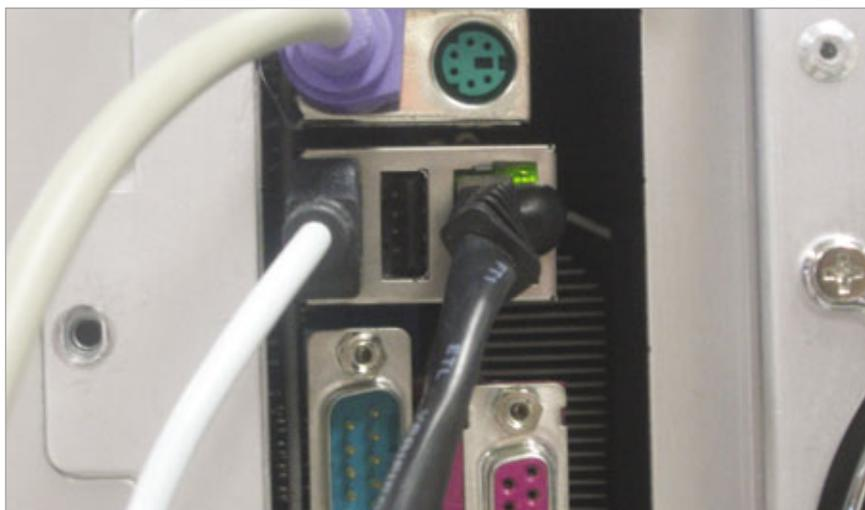
If you see error messages indicating a keyboard isn't present, it could mean your keyboard cable is unplugged, loose, or plugged into the wrong port. Most keyboards plug into a purple PS/2 port or USB port. Make certain the board isn't plugged into the green PS/2 port for mice.
