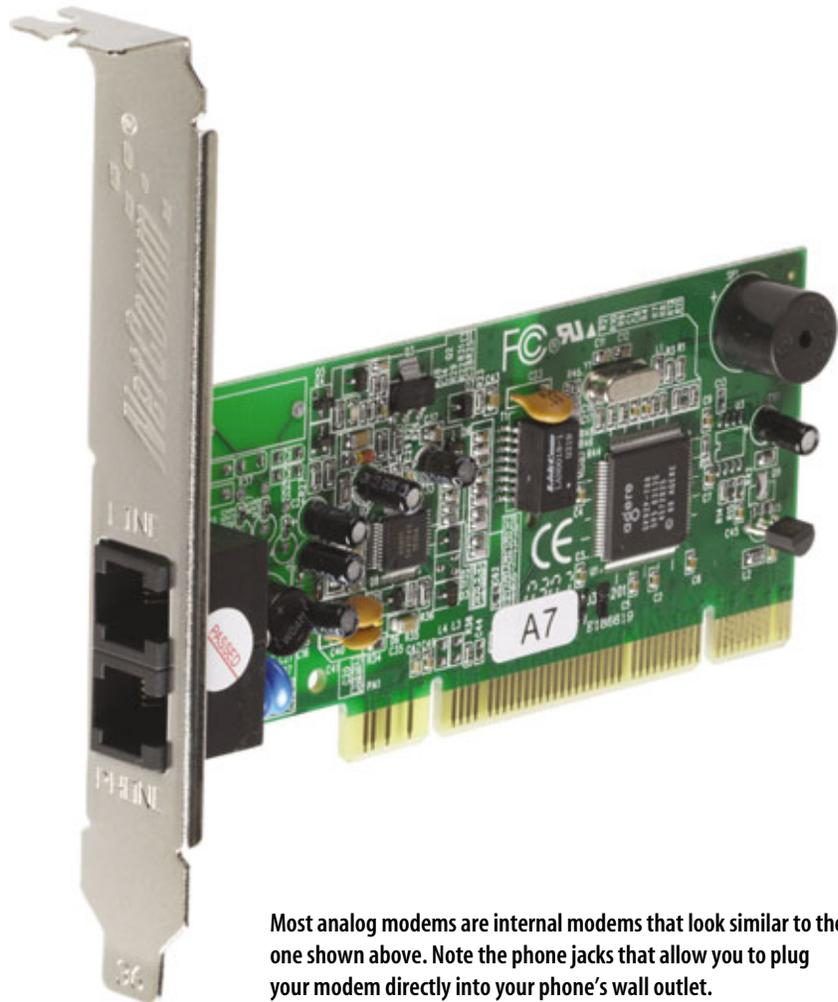
Most analog modems are internal modems that look similar to the one shown above. Note the phone jacks that allow you to plug your modem directly into your phone's wall outlet.
