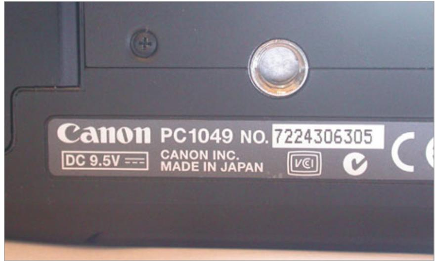
The serial number is usually located on the bottom of the camera.
