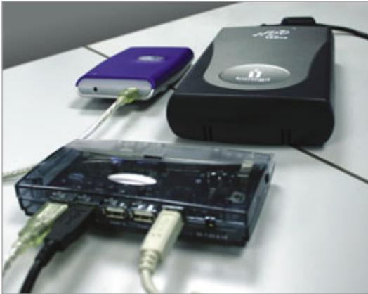
**External USB storage devices may not work when connected to a USB hub. If the drive isn't recognized, directly connect it to the computer's USB port.**
