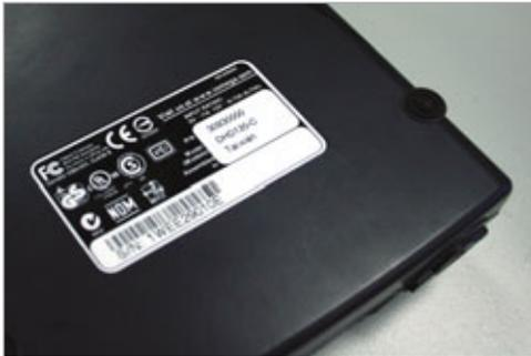
On an external hard drive, you can locate a drive's name, model number, or serial number above the bar code on the bottom of the drive.
