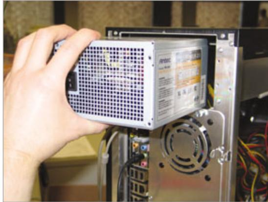
After you remove its retaining screws and disconnect all its power plugs, your power supply should slide out the back of the PC. Don't let the power supply fall into the case.
