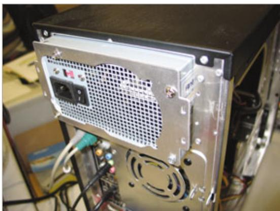
Four screws usually hold a PSU in place. However, this Lian-Li computer case uses an additional plate to mate the power supply to the case's rear panel.
