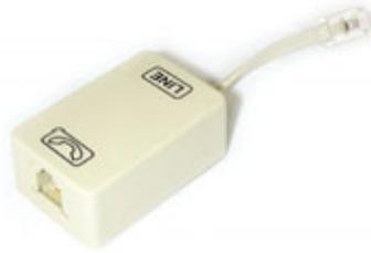
Installing an inexpensive DSL (Digital Subscriber Line) filter can get your MFD's (multifunction device's) fax component operational.
