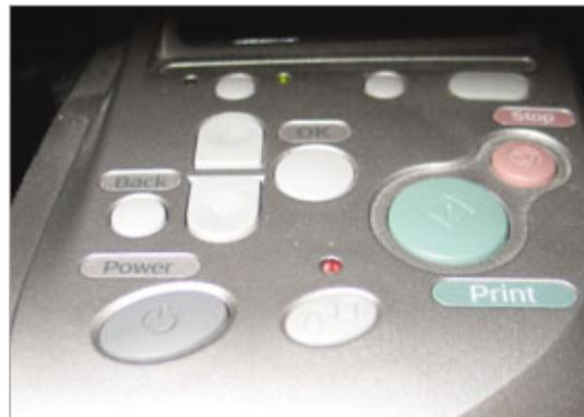
Most printers have an LED (light-emitting diode) that blinks when there is a printing error.
