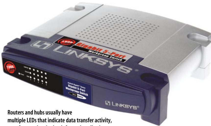
Routers and hubs usually have multiple LEDs that indicate data transfer activity, transfer speed and other information. Check out your manual to learn more about your device's lights.
