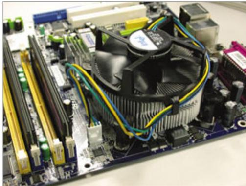
**Double-check the heatsink fan's motherboard connector before powering on your system if you've recently moved your PC or performed maintenance inside the case.**
