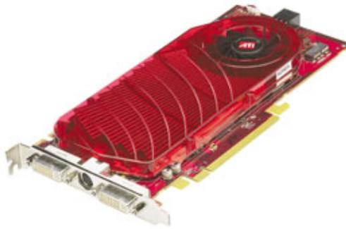
This graphics card from ATI requires a single 6-pin power connector from the PC's power supply.
