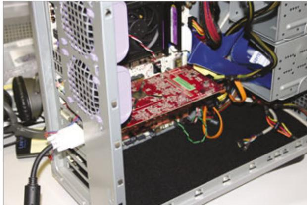
The graphics card is typically located in the top-most PCI (Peripheral Component Interconnect), AGP (Accelerated Graphics Port), or PCI Express slot on the motherboard, just below the CPU.
