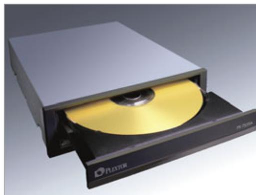
Most CD and DVD drives use the IDE interface. However, some Plextors (such as this PX-755SA) and Samsungs are SATA (Serial ATA) drives, and therefore don't have the jumper, cable, and DMA (direct memory access) mode issues that can crop up with IDE units.
