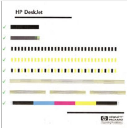
Most printers have one or more test pages (pictured is a color alignment test page) they can print to determine if things are working properly on their ends.
