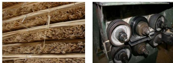
Figure 49: "crushing" des lamelles
