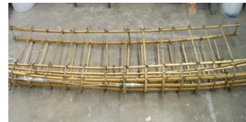
Figure 32: Armatures en bambou
