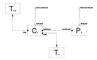
A class definition causes a class object and prototype instance to be created. The default delegate of the instance prototype is the Object prototype. The default super class of the class object is the Object class. Static members are added to the class object as fixed properties, and non-static members are added to the instance prototype as fixed properties. The internal references (traits, prototype, constructor, and delegate) between these objects are read-only.
