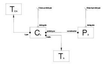
The illustration shows the shape of the class object that results from the following simple class definition:
