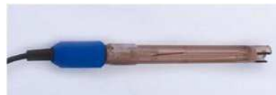
Photo 5: Electrode GE 105 (cliché GREISINGER ELECTRONIC, 2009)
