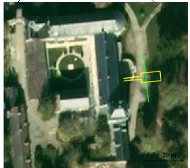
FIGURE 5.7: Location map of the study area. The limits of the underground room are represented in yellow. The geophysical profiles were acquired along the green line.
