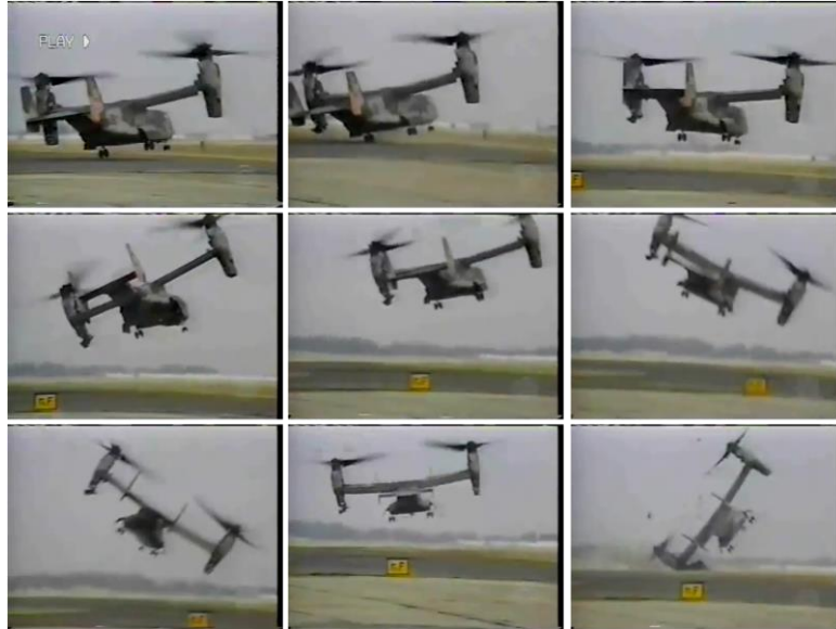
Figure 1-2. Roll oscillations during flight tests of Boeing-Bell V-22 tiltrotor from (DefenceVideos, 2013)
