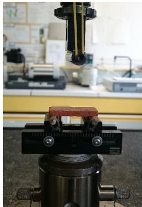
FIGURE 3.2.3 – Montage de flexion 3points
